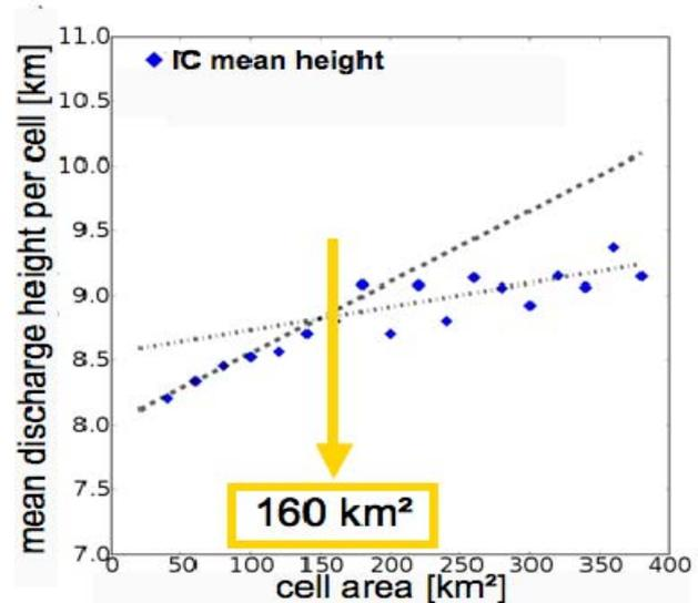
Statistical analysis of some 5000 LINET lightning cells in Central Europe: a single cell can grow up to 160 km<sup>2</sup> and shrinks thereafter; larger lightning areas contain more than one cell in different life cycles; from Meyer, V., "Thunderstorm Tracking and Monitoring on the Basis of 3D-Lightning (LINET) and Conventional and Polarimetric Radar Data", PhD Thesis, Physics Department, University of Munich, and DLR (Deutsche Luft- und Raumfahrt, Wessling, Germany), 2010.
