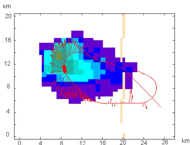
*The red arrow indicates the direction and magnitude of the horizontal field (maximum value ~12kV/m) at 6250m AMSL superimposed on the trajectory of the aircraft and the precipitation radar echo at about 2500m AMSL.*
