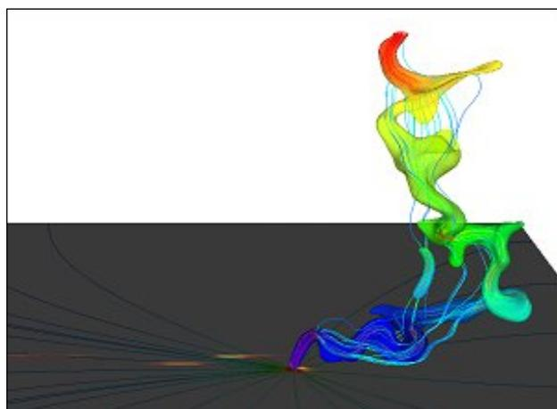
*Computation of a 6000K iso surface of a 50cm arc attached on a metallic plate. The electrical potential of the arc is color coded from 0 to ~400V.*
