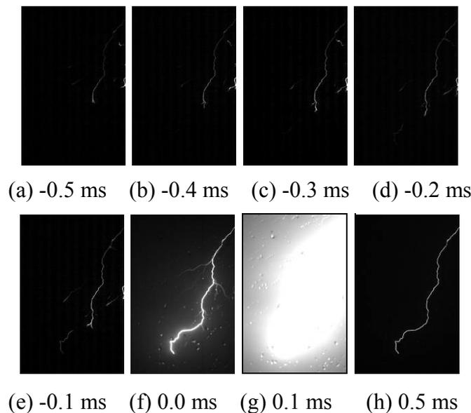
Fig. 1 High-speed camera records of L01. In frame a-e, luminosities are enhanced for a better view.
