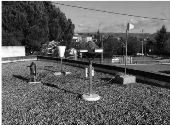
Left: HPicoNet multi measurement station over the roof of the Lavilledieu school (Ardèche). Right: Measurement of the electric charge of precipitation with a new induction ring.
