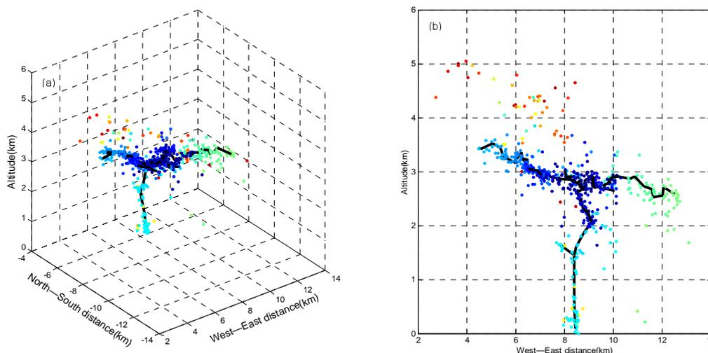
Fig.1 3D view (a) and north-southward vertical projection (b) of the channel created with our algorithm for a CG flash
