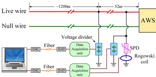
Fig.1 Schematic showing the measurement of induced voltage on the overhead power line.
