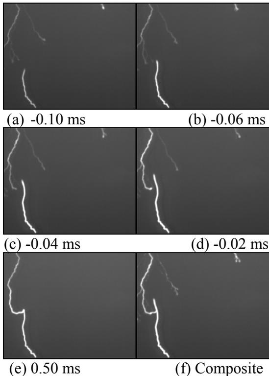
*Fig.1 High-speed images of F1111 captured by the high-speed camera with a sampling of 50,000fps. Fig. 1f is the composite image of 75 images before the return stroke and the image 0.5 ms after the return stroke.*
