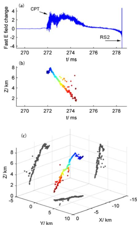
Fig.1 The 3D location of CPT occurred in –CG Case 6: (a) the fast E field change waveform, (b) the height of sources (Z) versus time, and (c) the 3D location and its projection on three coordinate planes (gray points).
