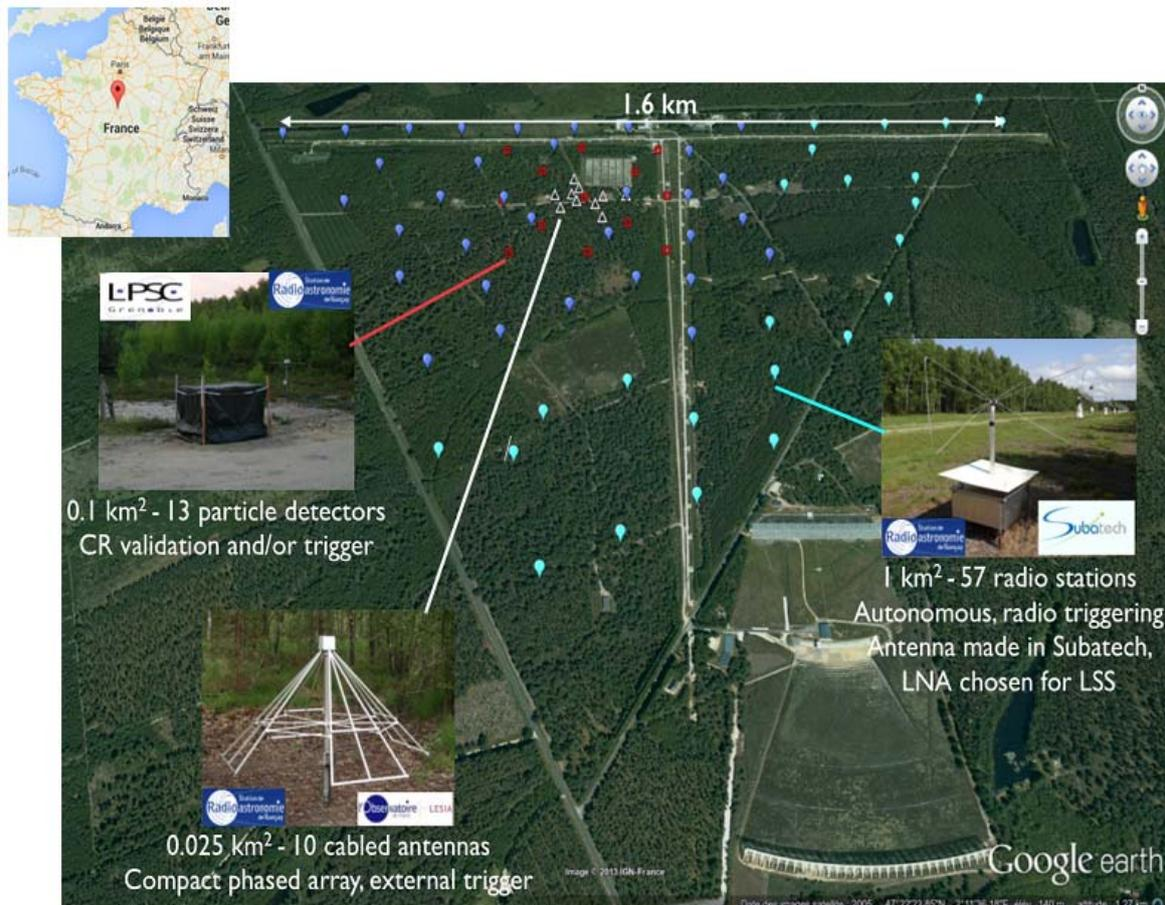
Figure 1 – General overview of the radio astronomy station in Nançay (see location in upper-left panel). We also present the various detectors of the CODALEMA experiment, dedicated to the observation of air showers initiated by high energy cosmic rays.
