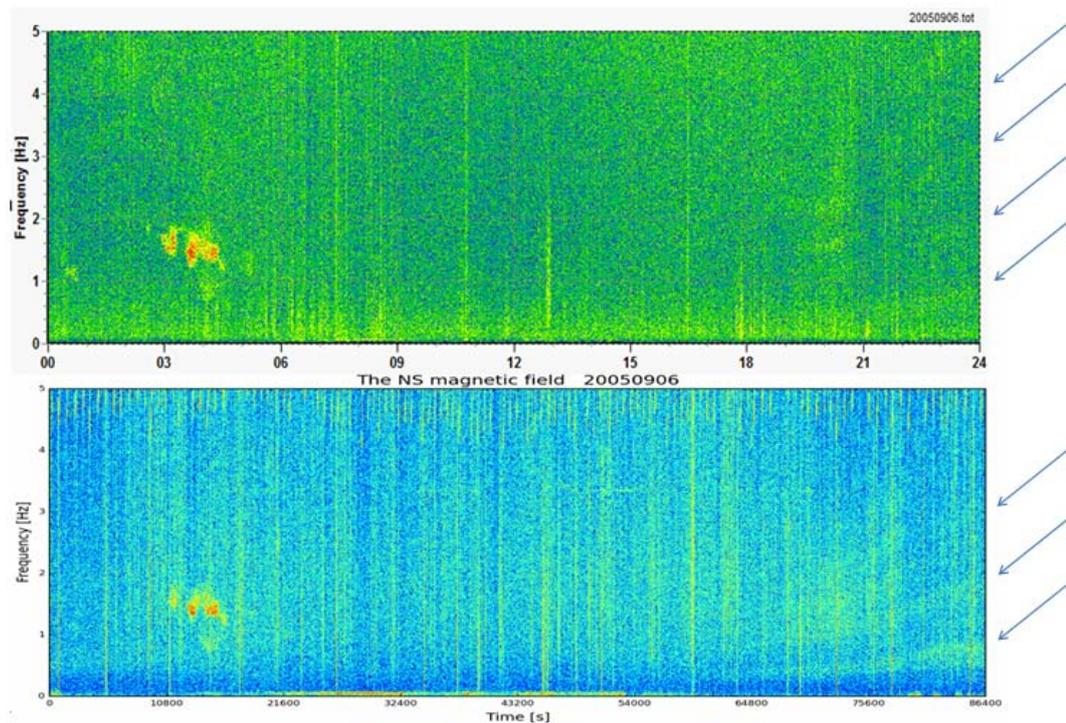
**Fig.1.** Dynamical power spectra computed from the horizontal magnetic field components recorded at the Hylaty station, Poland (top panel) and Nagycenk station, Hungary (bottom panel) for Sept 6, 2005 in the frequency range below 5 Hz. The common Pc1 pulsations in the morning UT hours (left portion of the plots) are readily identified. Ionospheric Alfvén resonances in the evening UT hours are indicated by arrows (on the right).
