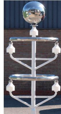
Fig. 1 The BTD-300 thunderstorm detector. The spherical and toroidal antennas are used to measure the electrostatic component of the E-field change due to lightning, wind-blown space charge and hydrometeor charge. The multiple antennas aid discrimination of different charge sources.
