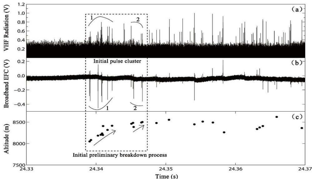
**Fig. 6** Negative CG flash 201124: (a) VHF radiation (relative value), (b) broadband electric field change (relative value), and (c) mapping altitude of the radiation sources.
