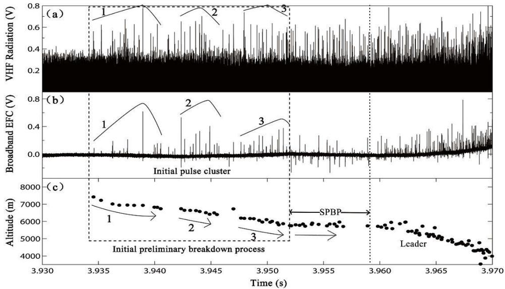
**Fig. 1** The initial preliminary breakdown process of negative CG flash 201503: (a) VHF radiation (relative value), (b) broadband electric field change (relative value), and (c) mapping altitude of the radiation sources.
