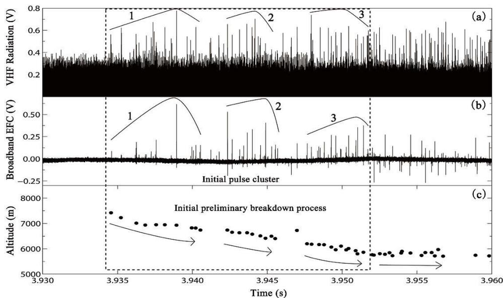
**Fig. 5** The synchronized charge of (a) the VHF radiation (relative value), (b) the broadband electric field change (relative value), and (c) the altitude of the radiation sources in negative CG flash 201503.
