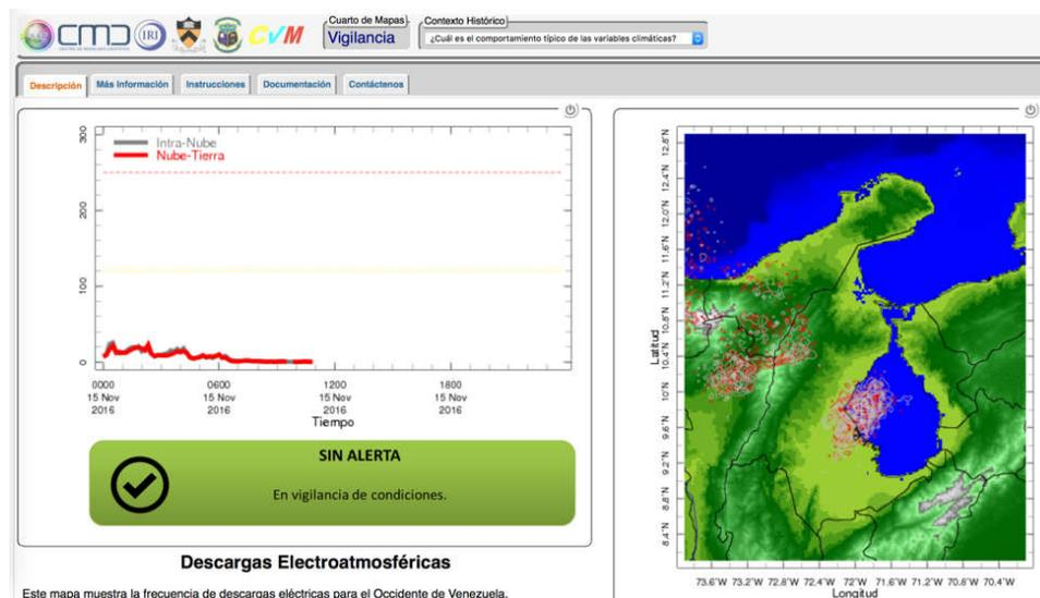
**Fig. 1** One of the products of SIVIGILA available in the Latin American Observatory Datoteca (see main text). The time series on the left shows the temporal evolution of intra-cloud (in grey) and cloud-to-ground (red) lightning in the Lake Maracaibo basin, shown in the right panel. For this day (Nov 15<sup>th</sup>, 2016) no warnings have been issued until noon: “Sin Alerta”.
