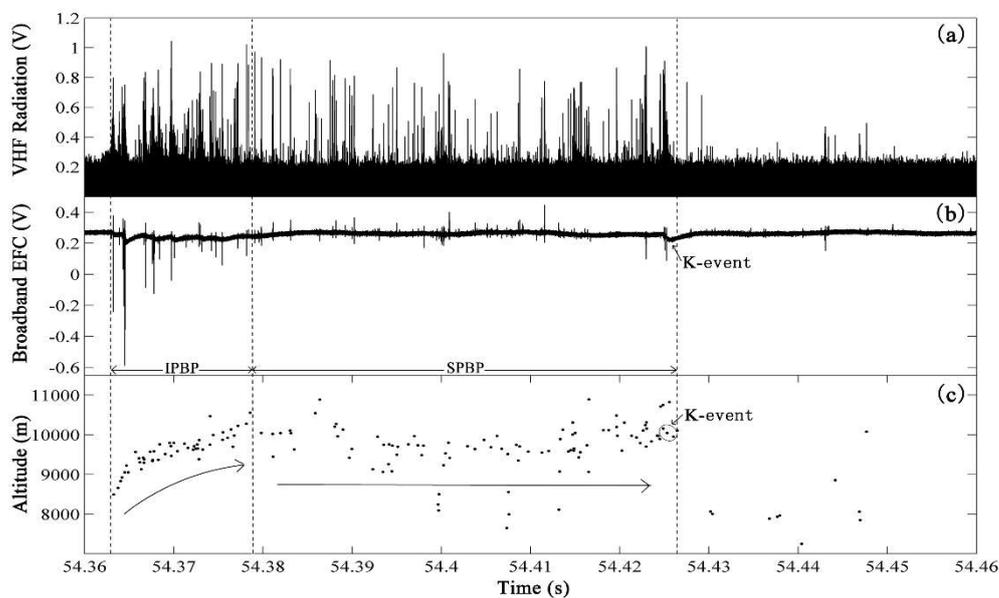
**Fig. 4** The preliminary breakdown process of the second category of IC flashes, showing the synchronized charge for the radiation sources in flash 210954 (54.36–54.46 s): (a) the VHF radiation (relative value), (b) the broadband electric field change (relative value), and (c) the altitude.
