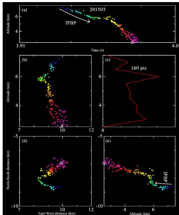
**Fig. 2** Radiation sources of the negative CG flash 201503 discharge: (a) height-time plot, (b) north-south vertical projection, (c) height distribution of the number of radiation events, (d) plan view, and (e) east-west vertical projection of the lightning radiation sources.
