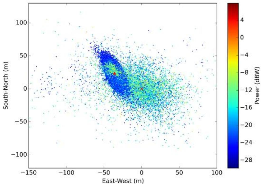
Fig. 1. Locations of corona discharges and the windmill (red cross) and the tower (red triangle). Color indicates radiation power.
