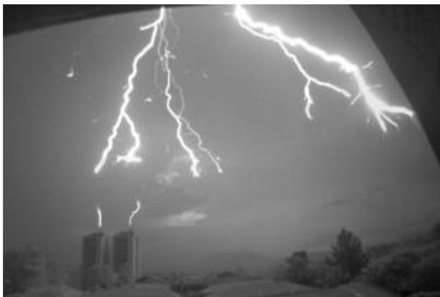
Figure 2 – Frame from high-speed video showing the upward connecting leaders from buildings in response to a negative CG flash (9 February 2014).
