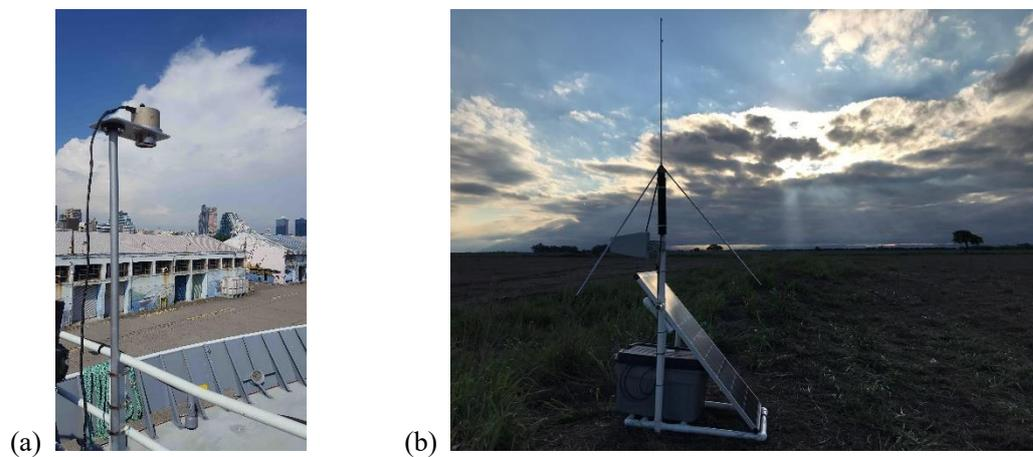
**Figure 1.** (a) Photo of EFM on the *R/V Thomas G Thompson* while in port in Kaohsiung, Taiwan (*credit: Timothy Lang*). (b) Photo of an LMA station installed near Monte Cristo, Argentina (*credit: Matt Wingo*).
